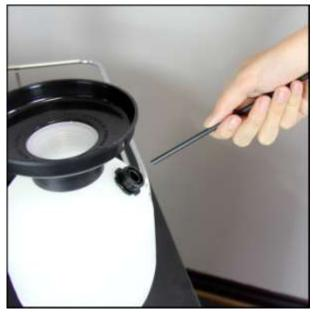
Insert Siphon Tube into Cleaning Bottle (1)
