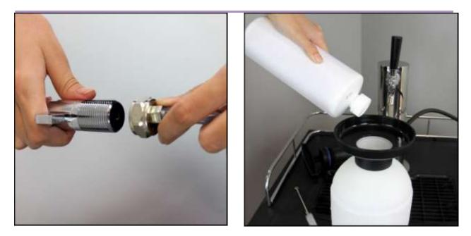
Attach the beer line to the Duplex Coupler. Pour the measured amount of the Cleaning Chemical (10) into the open Cleaning Bottle, following the manufacturer's specifications on the label. Add water as directed, ensuring not to overfill the container.
