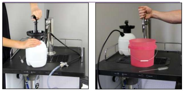
Unlock the pump handle by pushing down and turning the handle. Pump to pressurize the Cleaning Bottle. Place a bucket or pitcher under the faucet and open the faucet to allow the cleaning solution to flow through the line. Pump until dry. Rinse the Cleaning Bottle and fill it with clean, cool water and repeat the cleaning cycle to rinse the line of cleaning chemicals.
