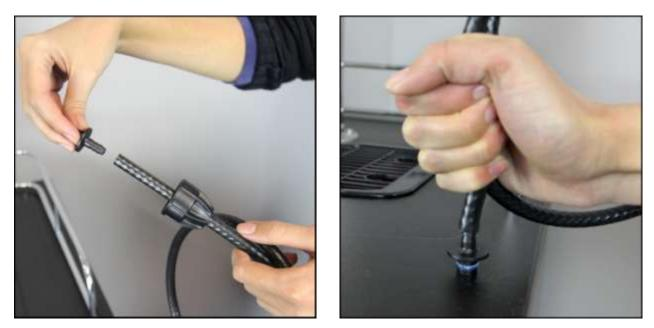
Insert Plastic Hose Barb (4) into Plastic Tube, pressing firmly until the flat portion touches the end of the hose. Use a hard surface to press down, if necessary.
