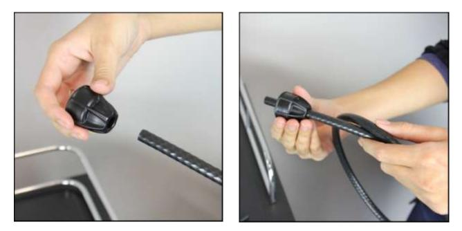
Slip plastic screw cap (7) onto 3/16" I.D. Plastic Tube (9), ensuring the flared end (larger opening) faces outwards.
