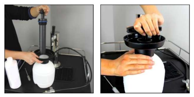
Insert the Pump (2) and twist to tighten. When inserting the Pump, the Siphon Tube can get in the way, pushing the Pump to the side. Be sure the Pump is straight up and down prior to twisting it in, so as not to cross thread the Pump.
