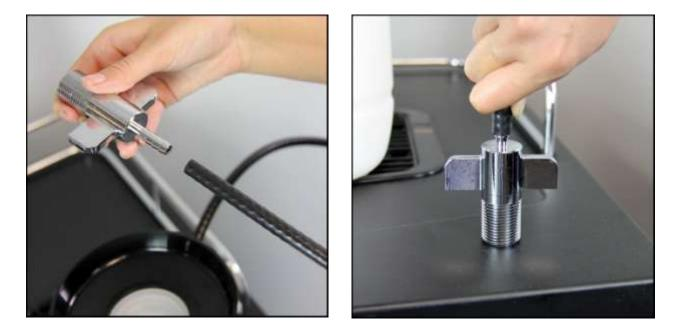
Insert the hose nipple of the Duplex Coupler (3) into the other end of the Plastic Tube. Press down on a hard surface until the tube touches the flat part of the Duplex Coupler.
