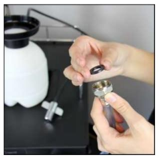
Make sure to keep the Neoprene Washer (5) in between the beer line fitting and the Duplex Coupler.
